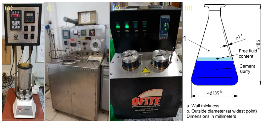
Fig. 2.11.: (a) API mixer, (b) pressurized consistometer, (c) atmospheric consistometer and (d) free fluid diagram.
