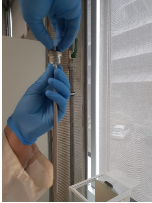
Figure 2.3.3: Assembly of a penetrometer with a cement sample
